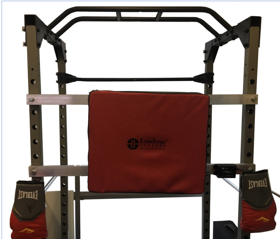
PunchSensor Installation: Mounted to an Exercise Frame
